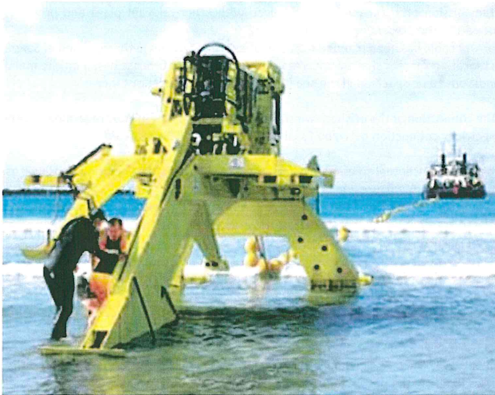
Photo 2. Illustrative photo of the plough which can be used for dredging the cable in the seabed.
