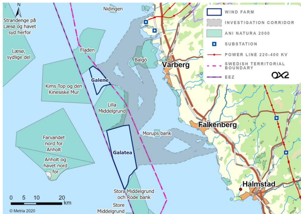
Figure 2. Overview of Natura 2000-areas and investigation corridors for connection cables (Source: The Swedish Environmental Protection Agency and Svenska Kraftnät (the Swedish TSO)).
