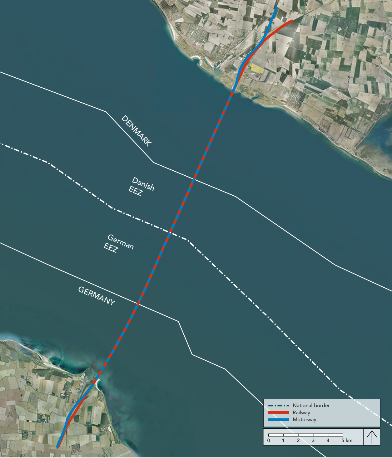
FIGURE 2 Conceptual design of an immersed tunnel – Alignment for the fixed link across the Fehmarnbelt
